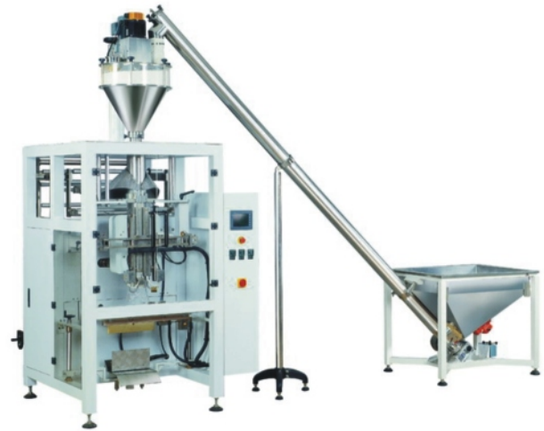
Form fill seal machine with screw feeder
